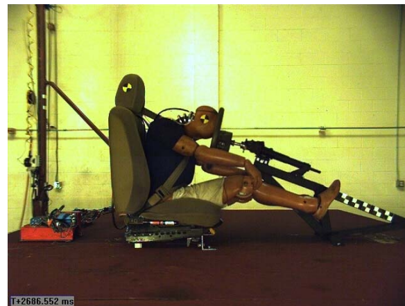
Figure 26. Hybrid III dummy with reduced musculature neck.
