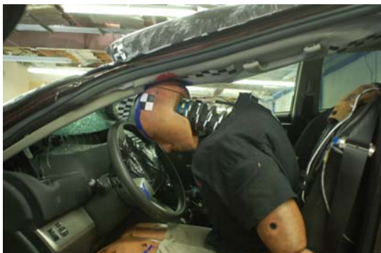
Figure 12. Soft neck of hybrid III dummy.
